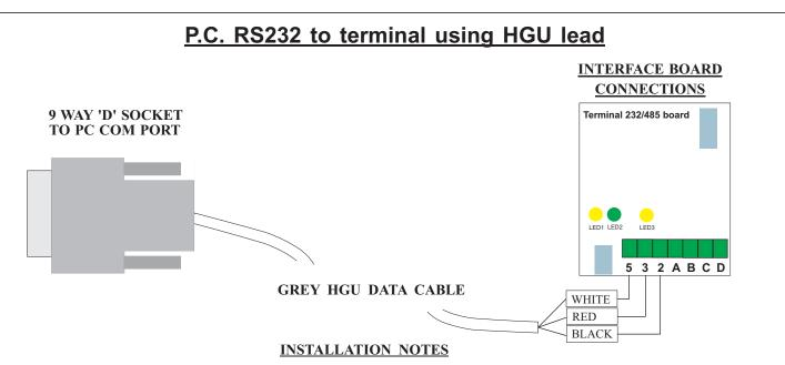
When wired correctly with the Computer and TP-1000 both switched on, LED's L1 and L2 will be lit on the Interface board. Green = TP-1000 OK, Yellow = P.C. OK. If this is not the case please check your connections.
